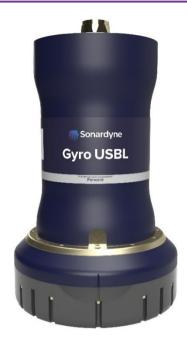
Gyro USBL combines a Sonardyne 6th (6G<sup>®</sup>) generation high performance HPT Ultra-Short BaseLine (USBL) transceiver and a Lodestar Attitude and Heading Reference System (AHRS) / Inertial Navigation System (INS) in the same mechanical assembly.
