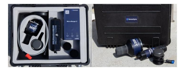
Micro-Ranger 2 has been designed as a true one box battery powered USBL solution, small enough to be carried as hand luggage on commercial flights and mobilised at short notice.
