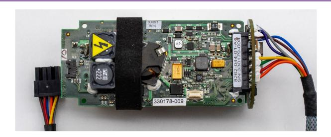
The AvTrak 6 OEM Nano Transceiver is a specially designed variant of the established AvTrak 6 for small underwater vehicles. It combines the functions of transponder, transceiver and telemetry link for intelligent subsea operations. It is available in OEM and Cabled form factors allowing for easy integration into many different platforms.
