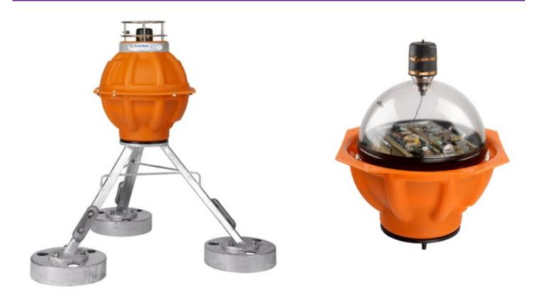
Fetch is a long-life subsea sensor logging node that enables data to be wirelessly extracted via its integrated high speed acoustic modem. It can be free-fall deployed to the seabed and will land in an upright position. This reduces deployment time and cost.
